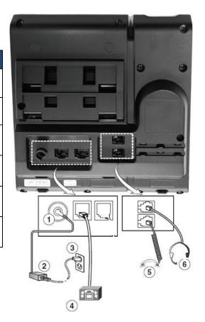
Notes: IP Phone 6921 cannot function properly when there is a failure in power supply.
